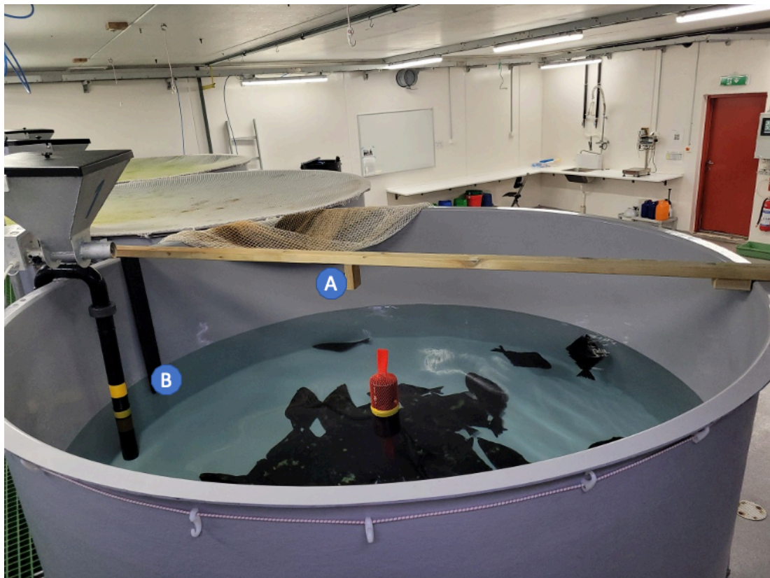
Figure 5: The camera rig pictured in a tank at the facility, with camera positions marked as A and B. Photo: Yvonne Rong, IMR.
