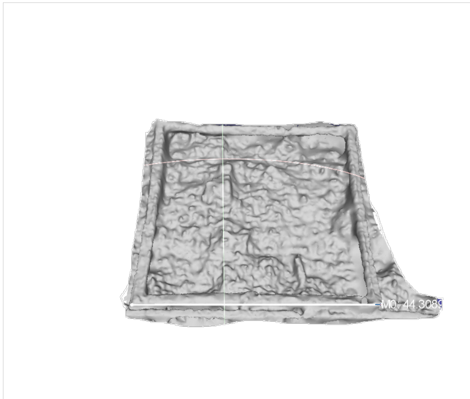
Figure 3.8: Measuring length of the 3D model using Meshlab to test the accuracy of the model.
