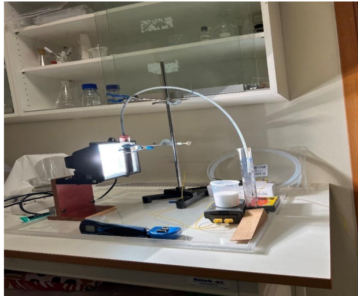
Figure 3.4 An image of the experimental setup for performing desalination using boiling and evaporation.
