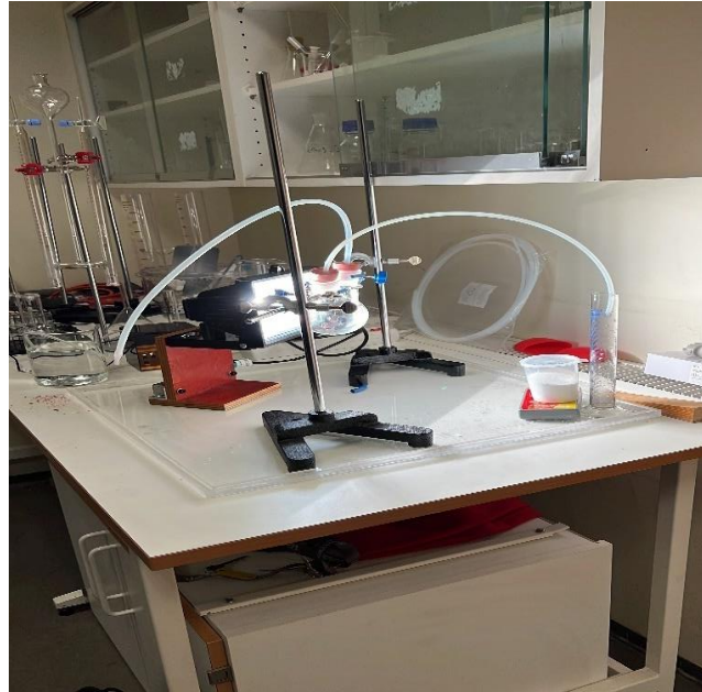
Figure 3.6 Image of experimental setup for desalination using boiling and evaporation which included a pump and round bottom flask.
