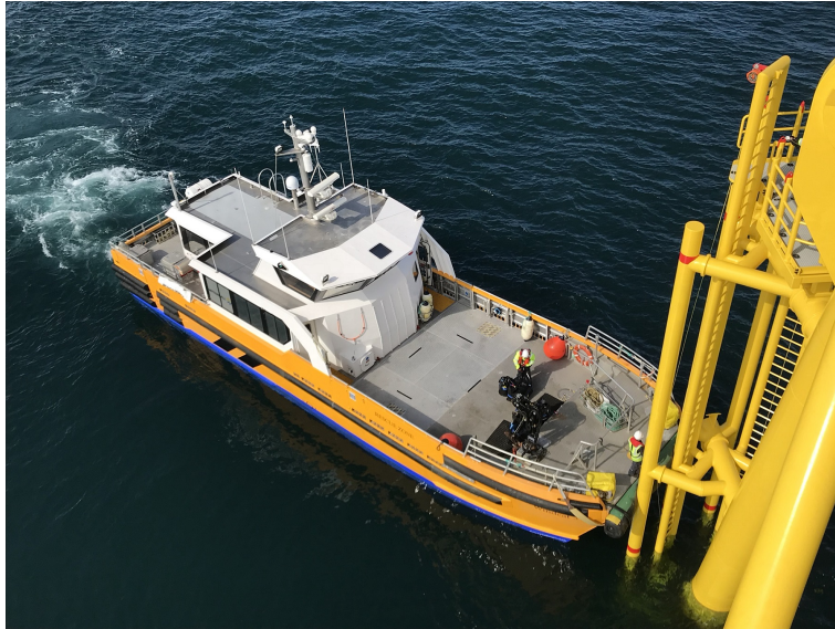
Figure 2: A crew transfer vessel disembarking technicians at an offshore wind turbine (photo: The Workboat Association [2]).
