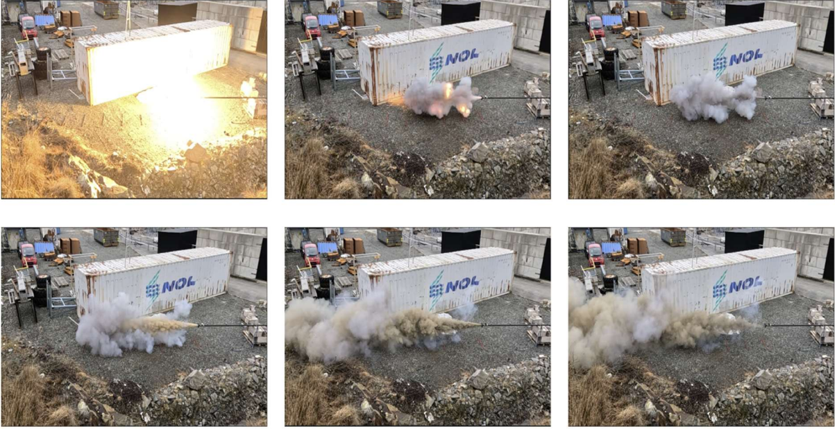
Figure 4-39: Collage of the flame and dust that escape the complete configuration during test number one.
