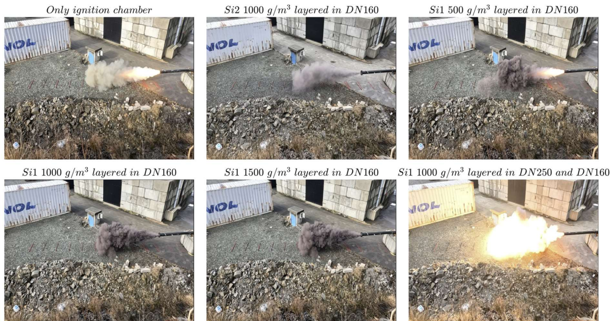
Figure 4-25: Ejected dust clouds and flames from the DN250/DN160 configuration. Notice the colors of the ejected dust clouds, the dark clouds indicate large amounts of unburnt dust.
