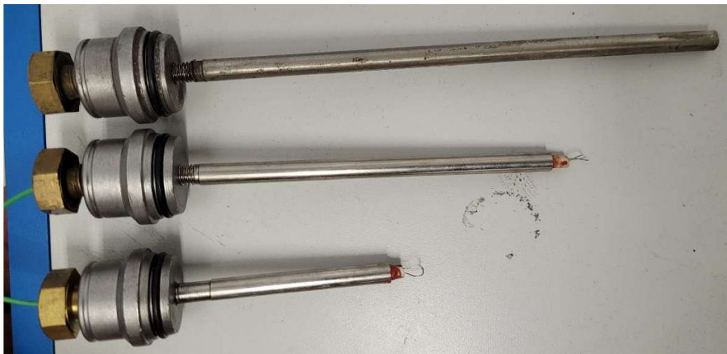
Figure 3-6: The different sizes of thermocouples, to reach the centre of the pipes.
