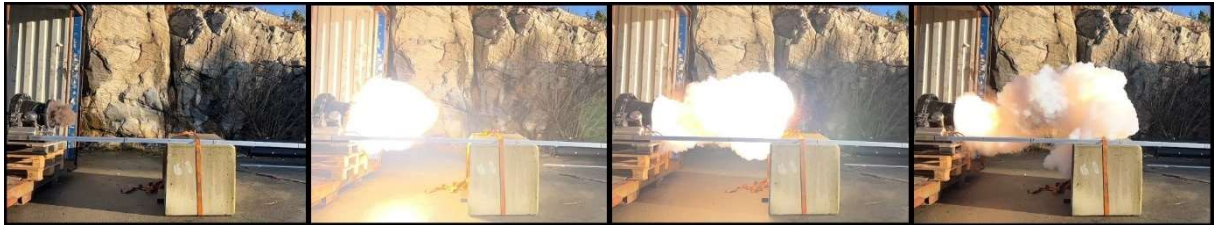
Figure 3-8: Ignition chamber test with 750 \text{ g/m}^3 Si-1 3 , corresponding to an amount of 24 grams.
