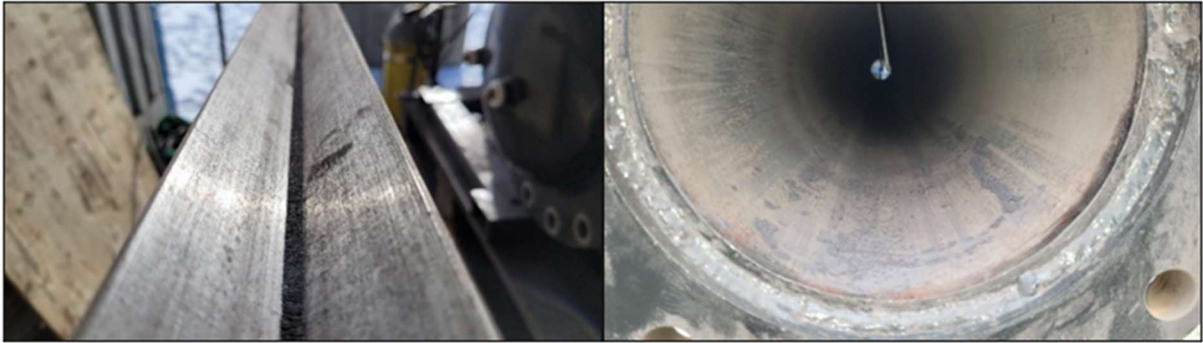
Figure 3-9: To the left; dust corresponding to a concentration of 250 \text{ g/m}^3 distributed in the largest angled iron, about to be inserted into DN160. To the right, DN160 with dust distributed on the inner surface.
