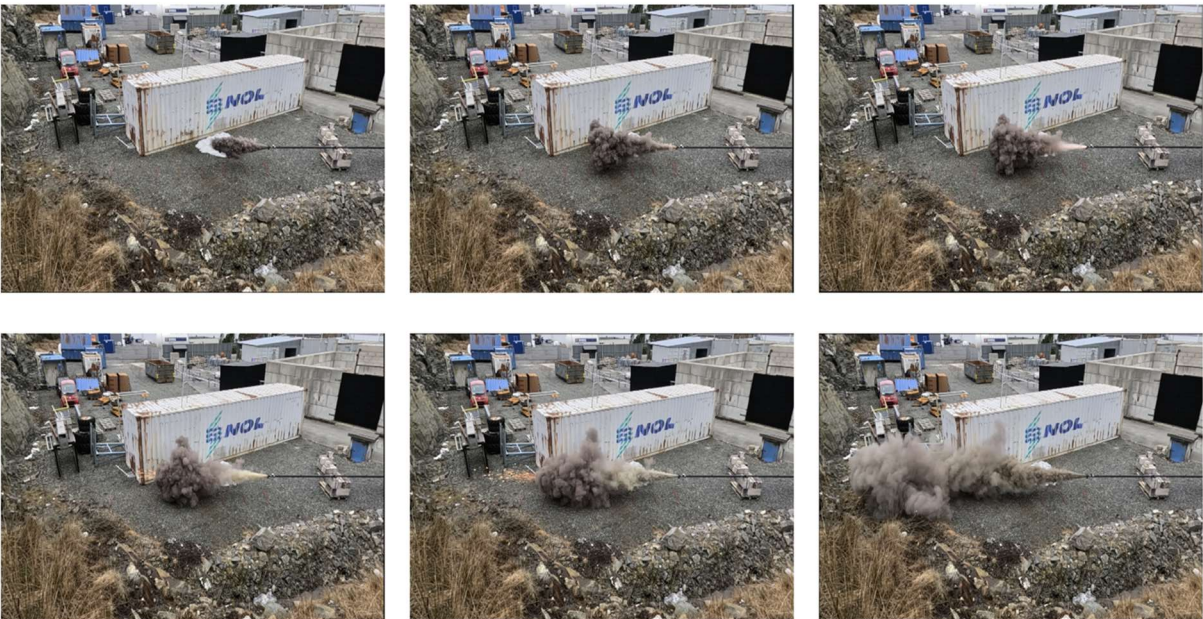
Figure 4-40: Collage of the dust that escape the complete configuration during test number two, it is difficult to percept the fire from the pictures, but some indications of flame exiting the pipe was distinguishable on the video.
