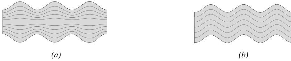
Figure 2.3: Modes in a vacuum-embedded steel plate. (a) Symmetric mode. (b) Anti-symmetric mode.
