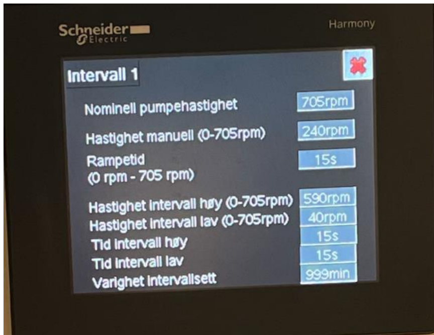
Figure 18. The screen of the PLC with the programmable options. The “Nominell pumpehastighet” (translated to Nominal pump speed) was the motors max pump speed.
