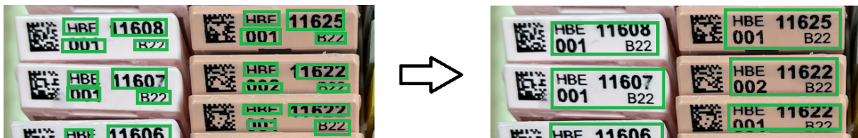
Figure 4.9: This figure shows how the algorithm merges the results from EAST to capture all the data on one cassette
