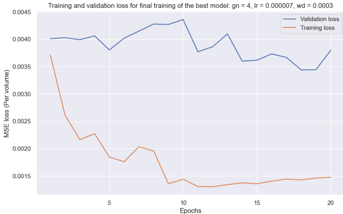
Figure 4.8: Training and validation loss of the model with the best-performing hyperparameters from the model selection. MSE = Mean square error, gn = Group normalization, lr = Learning rate, wd = Weight decay
