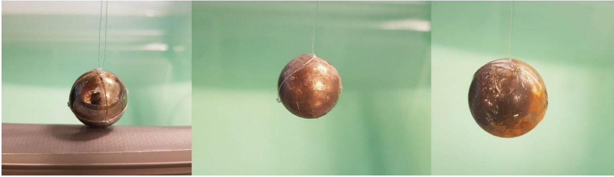
Figure 3.9: The three calibration spheres used, 22 mm tungsten carbide (left), 16 mm copper (centre) & 20 mm steel (right).
