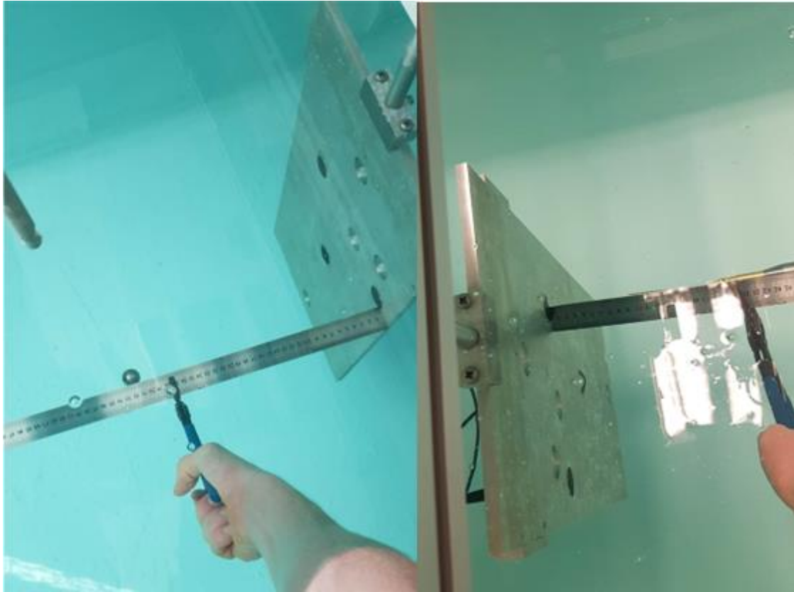
Figure 4.36: Finding absolute distance from transducer face to determine system delay using a ruler.
