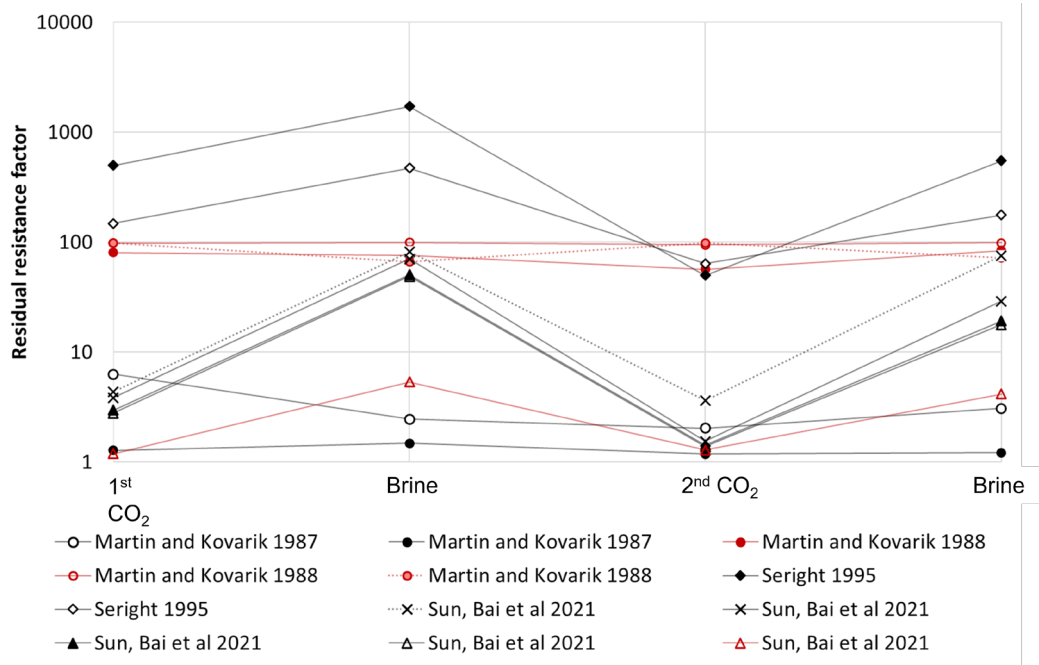
Fig. 2—WAG after CC/AP gel placement in sandstone. The x-axis starts at the first CO 2 injection. Multiple corefloods are presented in most papers (duplicate paper listings). The RRF values are provided in the appendix, Table A-2.
