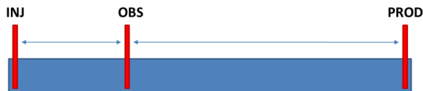
Figure 3. Crosswell Testing. For this testing method, an observer well between the injector and producer well is required to conduct a cross-well measurements.
