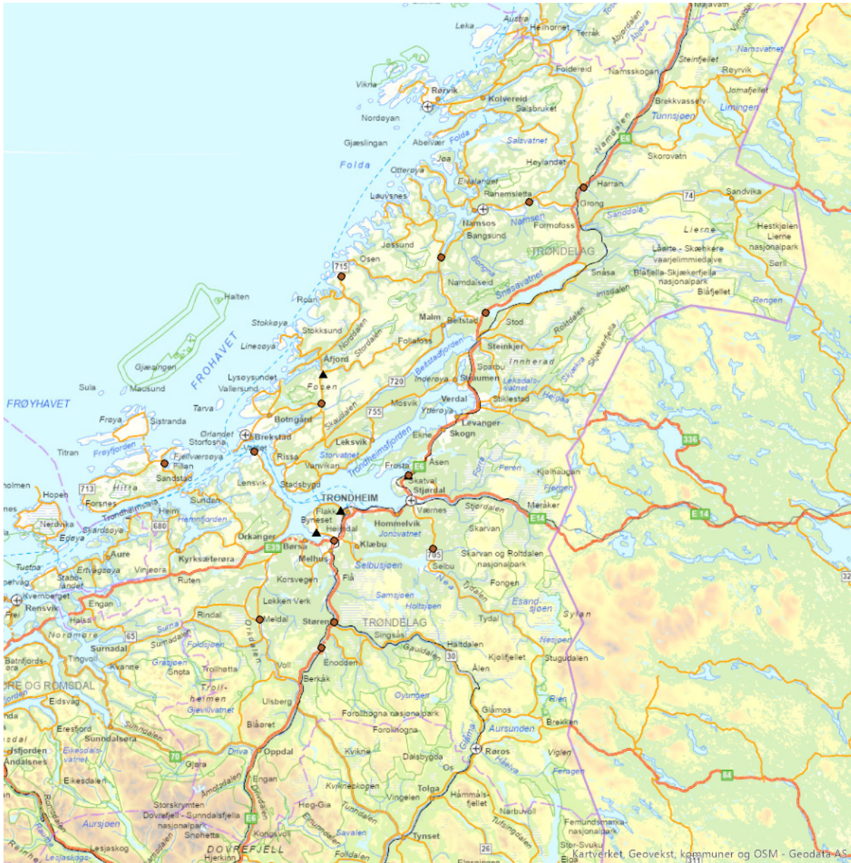
Figure 6.4: Charging facilities needed to cover Trøndelag county when not considering the impact of traffic. The locations marked with four triangles cover all routes when the range of a BEV is set to 400 km. The 14 circles are the needed facilities when the range is reduced to 250 km.
