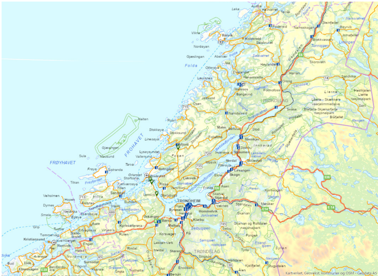
Figure 6.7: Existing charging facilities with one or more 150 kW chargers in Trøndelag county (blue markers) and additional charging facilities (green markers) needed to cover the whole county. The new charging facilities cover 50 paths, of the total 110494, that are not already covered by chargers with a power output greater than or equal to 150 kW chargers.
