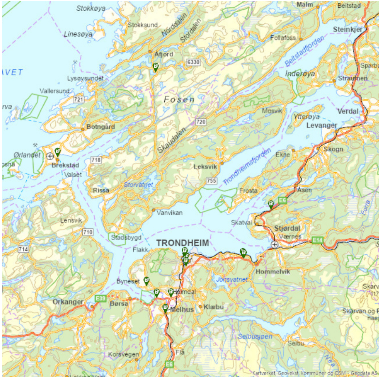
Figure 6.5: Charging facilities needed to cover Trøndelag county when accounting for traffic. A total of 13 nodes are chosen as charging facilities. The charging facilities are supplied with electricity from a total of 51 electrical substations.
