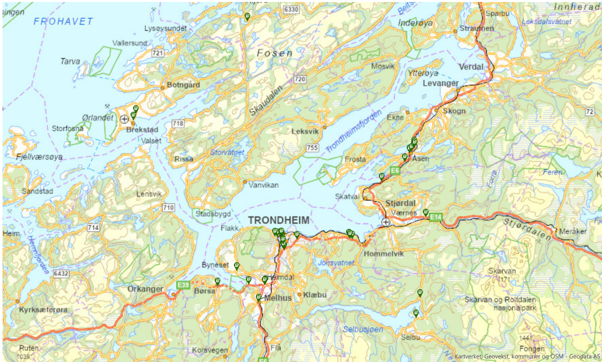
Figure 6.6: Charging facilities needed to cover Trøndelag county when accounting for traffic. A total of 43 nodes are used for charging facilities. Each node is only supplied by one electrical substation. The charging facilities are supplied with electricity from a total of 43 electrical substations.
