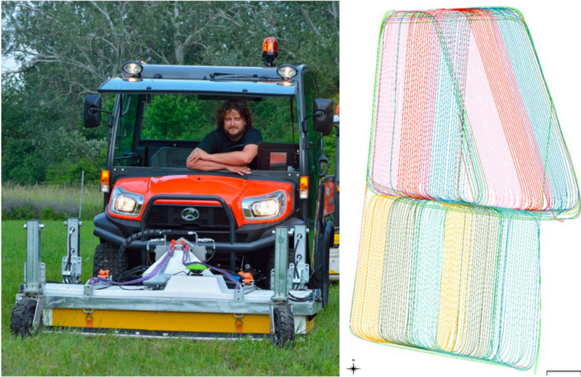
Figure 2.7: Illustration of how a GPR setup to the left, with the swath pattern to the right. Modified from (Trinks et al., 2018)
