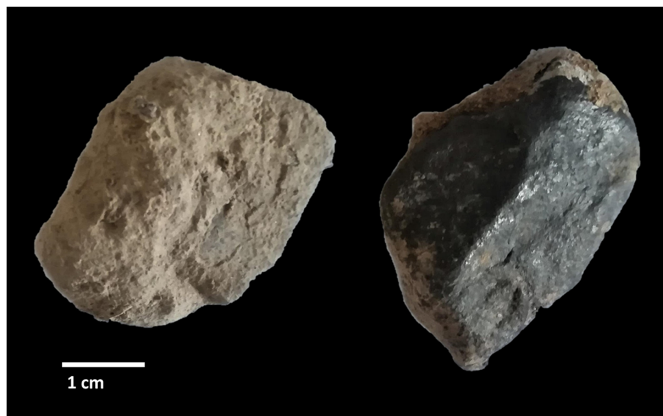
Fig. 2 Hydrochloric acid treatment of specular hematite. OBP specular hematite piece with calcium carbonate concretions. Left: before acid treatment. Right: after acid treatment
