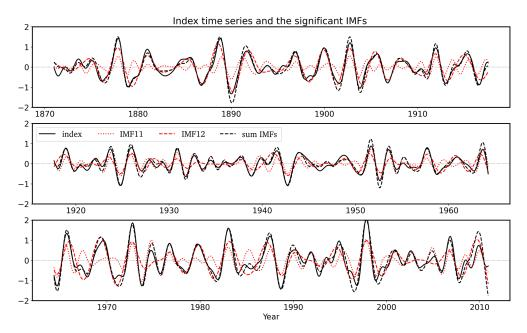
**Figure 3.** Time series (1871–2010) of the Niño3 index from IMF 11 (red dotted line) and IMF 12 (red dashed line) obtained via MEMD. The sum of the two IMF indices (black dashed line) and the band-pass-filtered (16–53 months) Niño3 index (black solid line) are also shown. All data are standardised.
