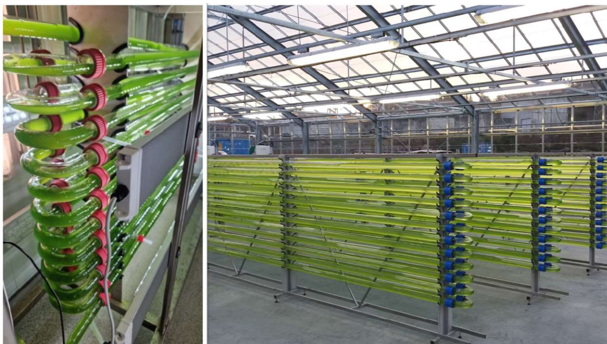
Figure 4. 16: The microalgae Nannochloropsis is cultivated in bubble columns before inoculation in 25 L photobioreactor (left) ultimately reaching the NAM750 reactors (right). Photo: Jeroen de Vree.
