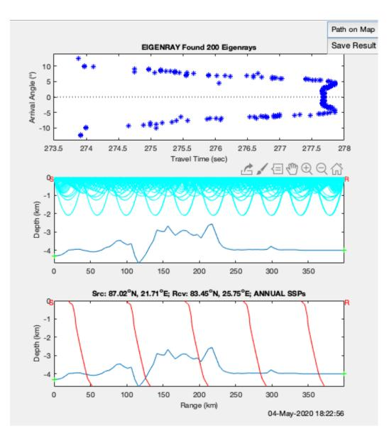
Figure 2.3: The three panel visualization of results from Eigenray. The upper panel contains arrival angles for each path, the middle panel shows the ray paths of the eigenrays and the bottom panel shows the SSPs for the path.
