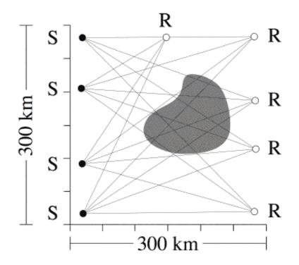
Figure 2.1: Acoustic tomography with four sources (S) and 5 receivers (R), giving 20 different acoustic paths[1].
