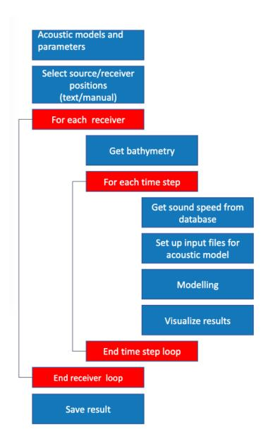
Figure 5.3: An overview of how the plotZRT-file handles several receivers and time steps.
