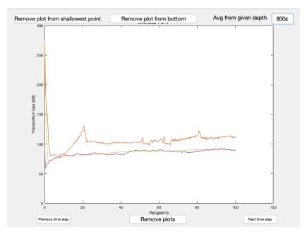
Figure 6.17: The average transmission loss on a path from the surface to a given depth (here 800 m), to a the shallowest point on the path and to 4500 m.
