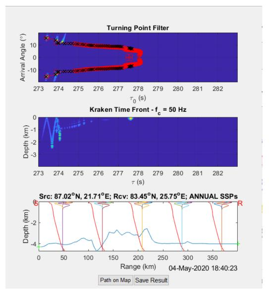
Figure 2.5: Krakens three-panel plot. The upper plot contains a turning point filter, the middle plot displays the time-fornts and the bottom plot contains SSPs.
