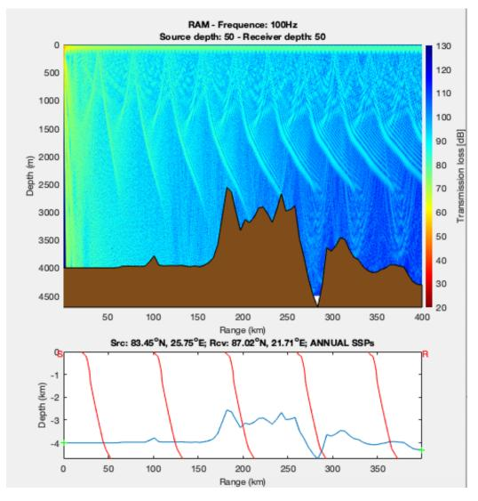
Figure 2.6: Visualization of results from Ram. It's a two panel plot whereas the upper plot shows the transmission loss, and the bottom panel shows the SSPs.
