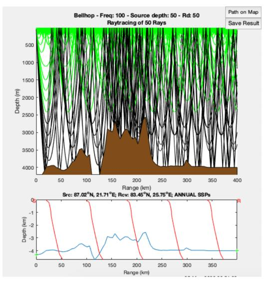
Figure 2.7: This is one of the possible results from running Bellhop. The upper panel shows the ray paths, while the bottom plot shows the SSPs.
