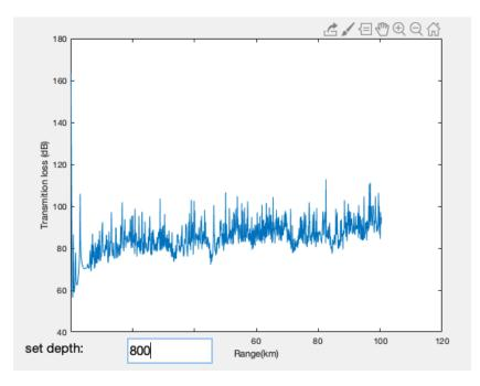
Figure 6.16: The transmission loss on a given depth as a function of range.
