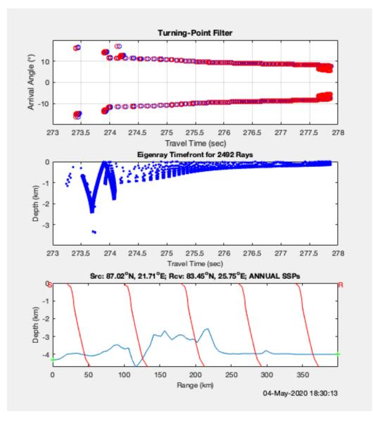
Figure 2.4: The three panel visualization of results from Eigenray with time fronts. The upper panel contains information about number of turning points for each path, the middle panel shows the eigenrays time fronts and the bottom panel shows the SSPs for the path.
