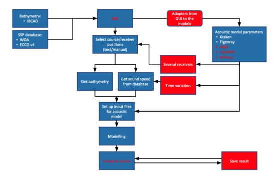
Figure 5.2: Block diagram of the Arctic package after adding more models, saving and other functionalities.
