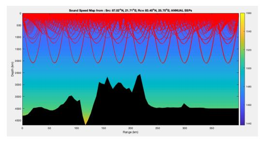
Figure 6.15: The eigenrays plotted on top of the sound speed profile. Bathymetry shown in black.
