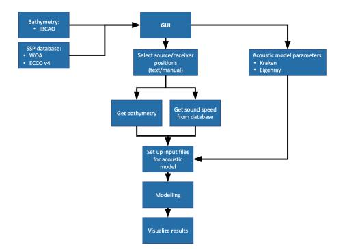
Figure 5.1: Block diagram of the original version of Arctic package.
