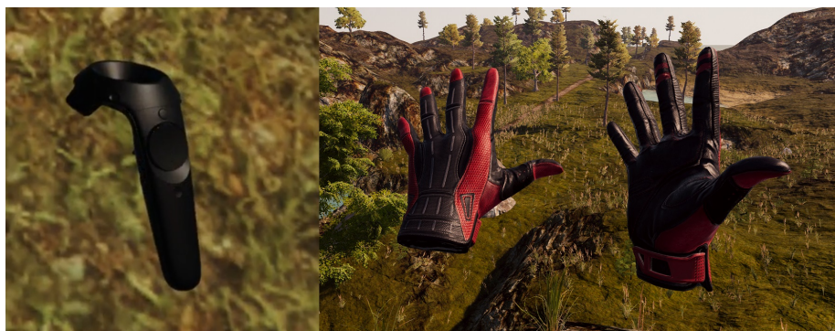
Figure 3.6: On the left: the controller representation utilized in VR Walk BSc, an interactive model from the SteamVR plug-in featuring all buttons present on the physical controller. On the right: The controller representation currently used. Hand models from the SteamVR plug-in that animate in response to controller input and can be manually posed.
