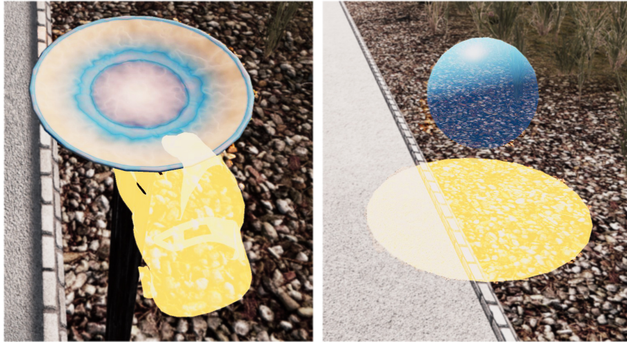
Figure 3.23: The left image shows the outline of a hand, instructing the player to grab the plate. The right image shows the player where the plate must be held to receive a balancing ball. When the plate is held in the correct position, the ball becomes solid and the physics engine takes control of it.
