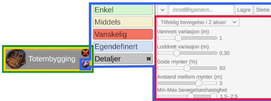
Figure 3.32: The nested composition of a path builder button. Green : Click-and-drag slot area, Yellow : Main body of the button, Blue : The common elements of the configurable buttons, Red : The activity-specific settings.
