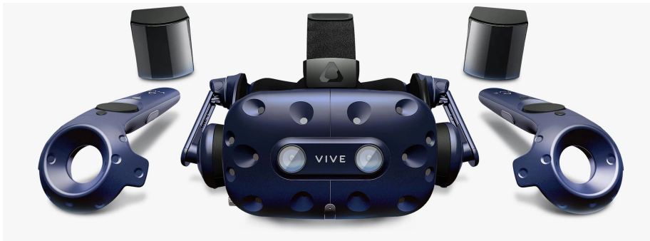
Figure 2.1: An example of fully immersive VR hardware; the HTC Vive Pro with controllers and base stations for the Lighthouse tracking system. During the development of VR Walk: Game, this was the model most frequently used. Photo: HTC Corporation.
