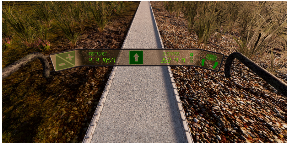
Figure 3.8: The treadmill front panel, featuring buttons for increasing and decreasing movement speed on the left, a start/stop button at the center, and a statistics field and safety indicators on the right.
