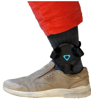
Figure 3.1: A HTC Vive tracker strapped correctly to the player's ankle. Also pictured is one of the shoes used as reference for the virtual representation of the player's feet.
