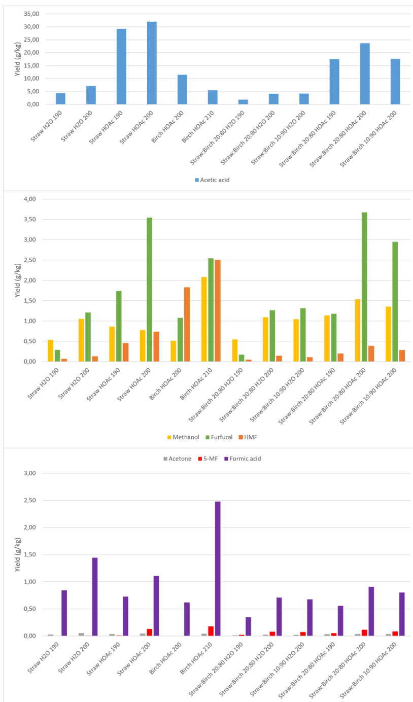
Figure 4.615: The total yields of identified organic compounds found in side streams from steam explosion of hardwoods and agricultural waste materials. Figure is taken from Hermundsgård et al. (manuscript)
