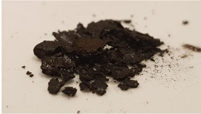
Figure 8: Black particles created from polymerization of furfural.
