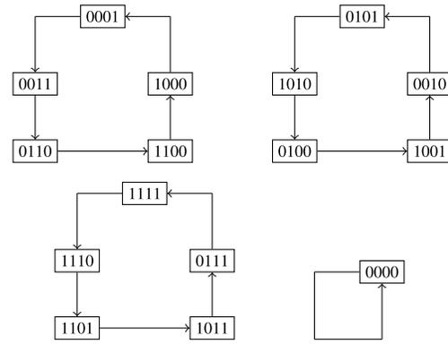
Fig. 1. The state diagram of the 4-stage LFSR.
