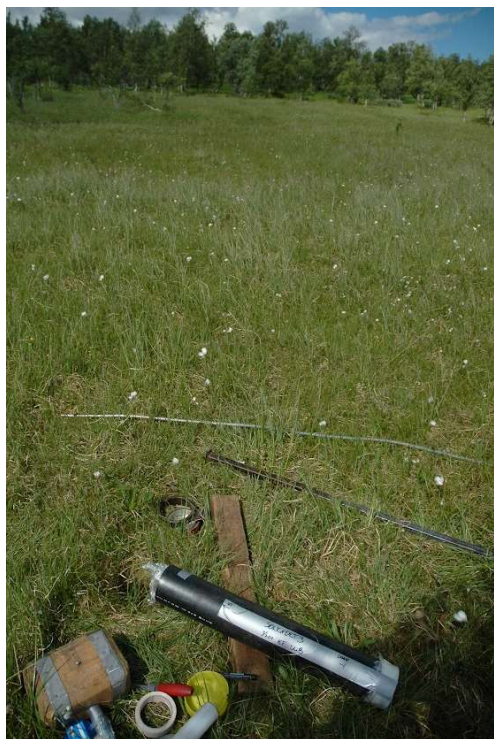
Figure 12. The peat core collection equipment, with a black plastic tube containing the peat core sample, located in rich-fen vegetation in Sølendet.
