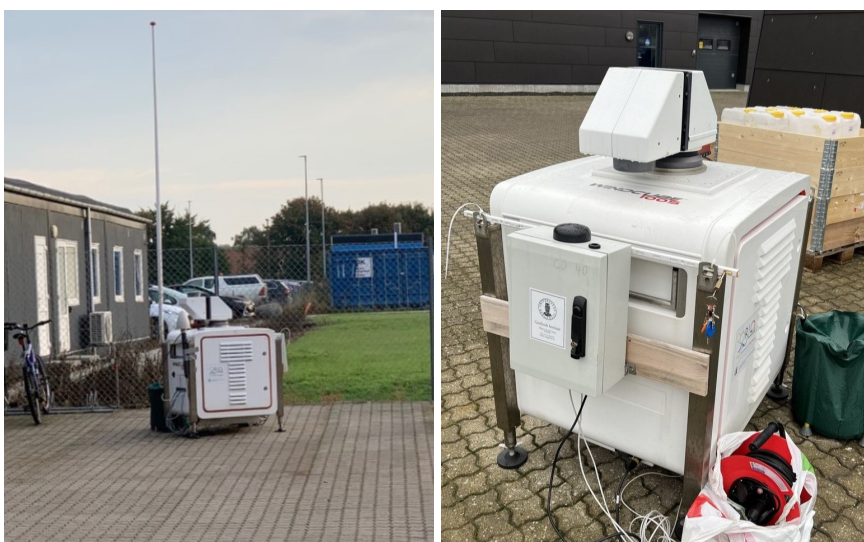
Figure 3.4: Leosphere WindCube 100S placed at Rødby harbour (photo courtesy of Shokoufeh Malekmohammadi).
