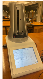
Figure 1: The spectrometers used in this study. Nanalysis 1.4 T (60 MHz) benchtop NMR spectrometer (left). Bruker AVANCE NEO 14.1 T (600 MHz) vertical bore NMR spectrometer (right). 5 mm (o.d.) tubes with a sample volume of 0.6 mL are used on both spectrometers.
