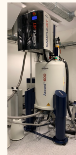
Figure 1: The spectrometers used in this study. Nanalysis 1.4 T (60 MHz) benchtop NMR spectrometer (left). Bruker AVANCE NEO 14.1 T (600 MHz) vertical bore NMR spectrometer (right). 5 mm (o.d.) tubes with a sample volume of 0.6 mL are used on both spectrometers.
