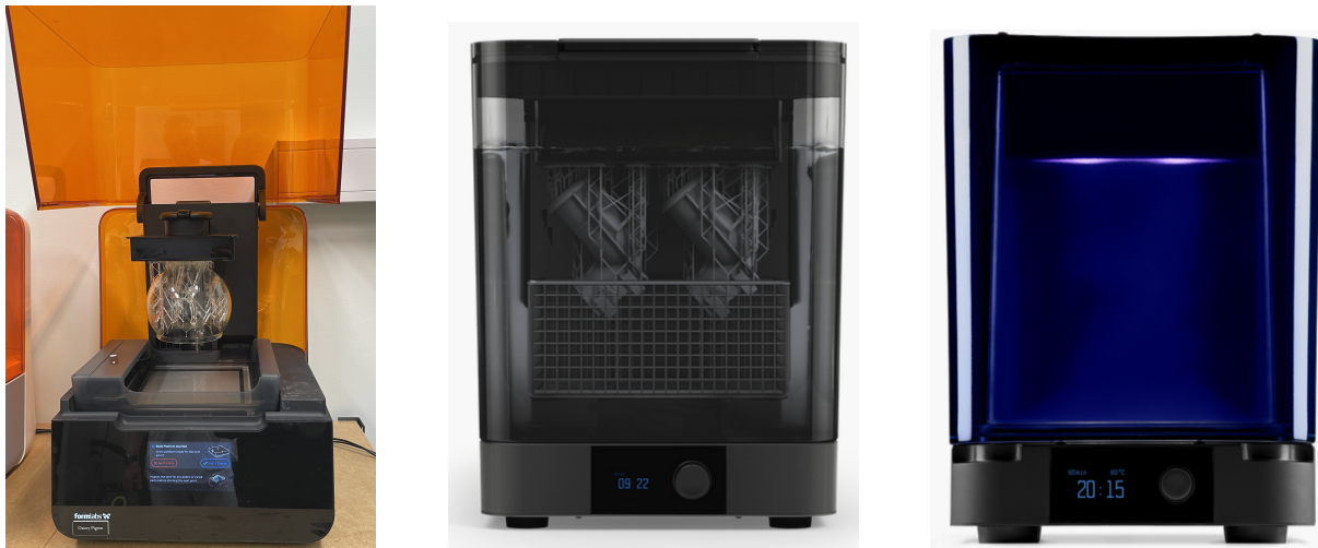
Figure 3.6: Picture of the Form 3+ 3D-printer with the printed phantom, the Form Wash [21] and Form Cure [21].
