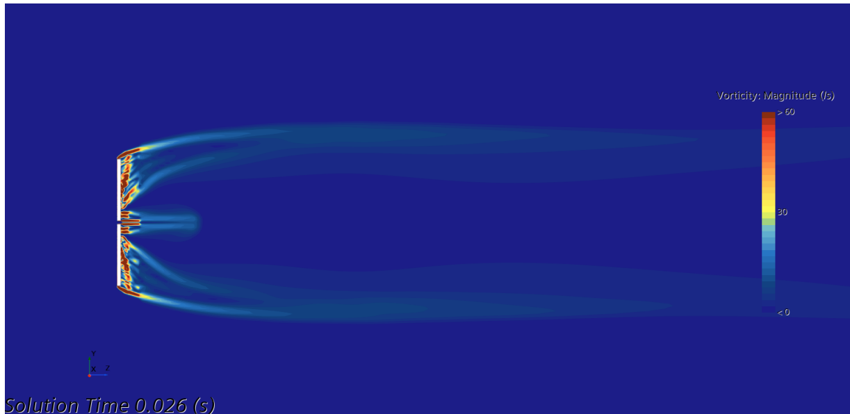
Figure 3.25: Vorticity field from the reference Detached Eddy Simulation on the actual geometry of the porous disc which will be used for comparison against results obtained through CFD RANS simulations.
