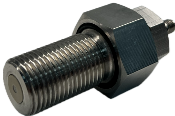
Figure 5.1: Picture of the coaxial probe antenna used for the experiments.
