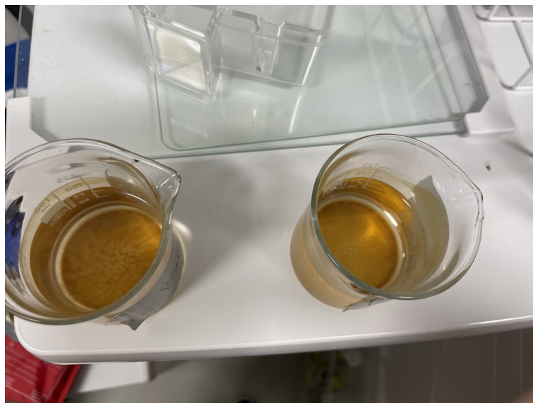
Figure 3.6: Samples. Left samples is from the bypass and the right sample is from the tank
