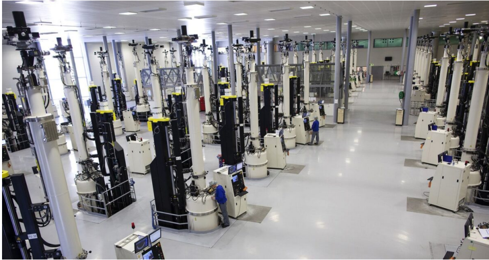
Figure 1.2: The Czochralski puller area in NorSun's factory. [1]
