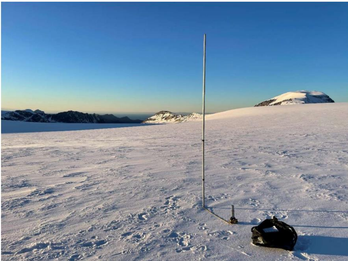
Figure 2.5: An ablation stake used in glaciological method on Engabreen. The markings on the pole are used to determine elevation change of the glacier surface (figure from Andreassen, Elvehøy, & Kjølmoen, 2023).
