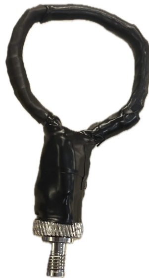
Figure 4.11: Homemade single-loop probe – Magnetic field probe made to the specifications of Douglas C. Smith [108], to measure the resonance frequency of the enhancing coil. Components used to make this were a BNC to SMA connector, heat shrink tubes of various sizes, solder, copper snail tape, and tinned copper wire.
