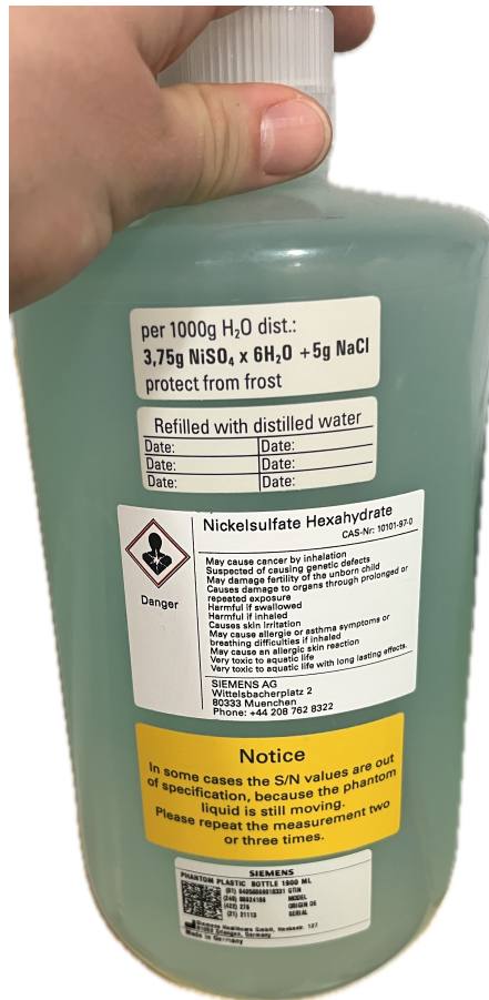
Figure 3.7: Picture of the chosen MRI phantom – This phantom produced by Siemens Healthineers contains a liquid solution of 3.75\text{g NiSO}_4 \times 6\text{H}_2\text{O} + 5\text{g NaCl} per 1000\text{g H}_2\text{O} and was used for coil loading during laboratory tests and phantom imaging.
