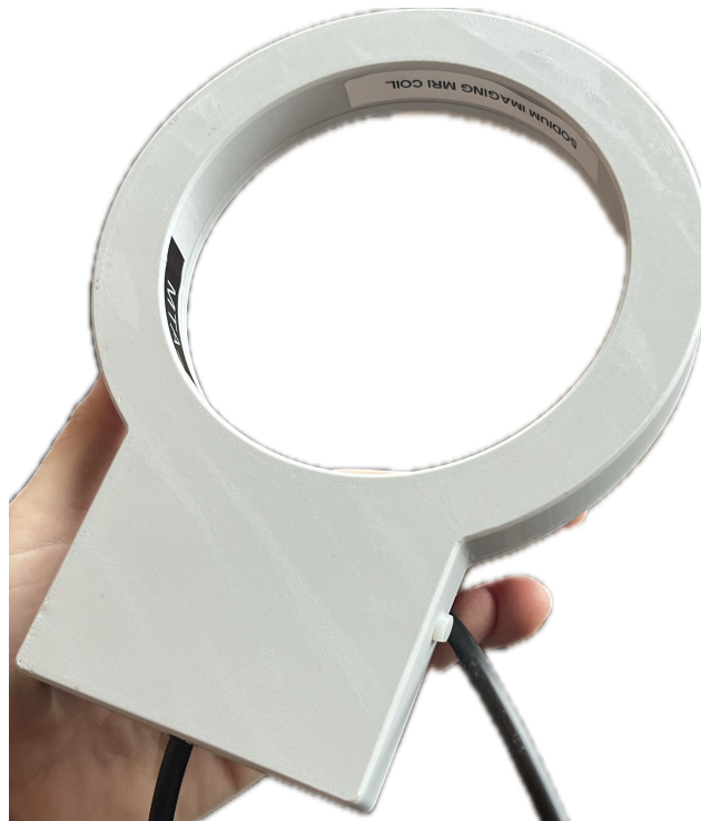
Figure 3.6: Picture of the Prior Design Two surface coil
