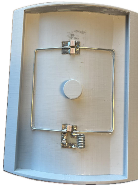
Figure 4.10: Image of the enhancing coil – The final enhancing coil mounted on the 3D printed enhancing holder.
