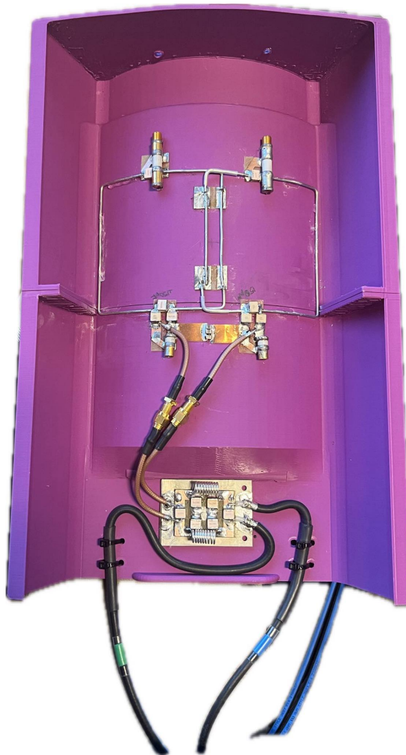
Figure 4.13: Image of the quadrature coil – The final electrical design of the quadrature coil mounted on the 3D printed stand-alone coil holder.
