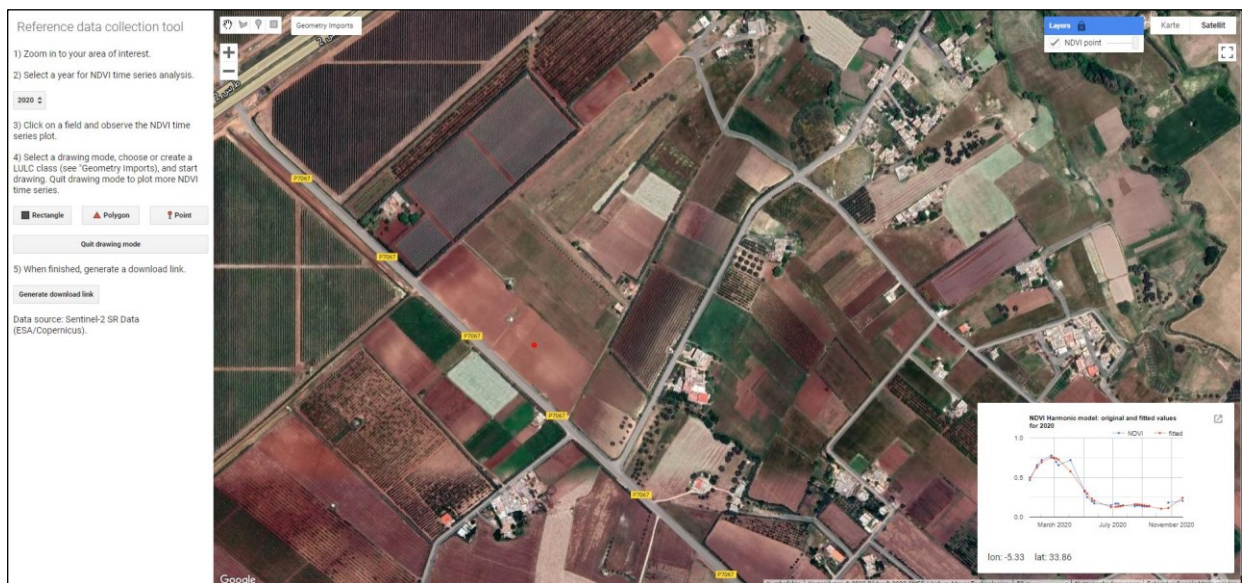
Figure 3. Reference data collection tool using NDVI time series inspector developed in GEE with S2 NDVI TS and harmonic fit based on GEE's implementation example [60]. Per click time-series information allowed for categorizing annual crops into "winter", "spring", "summer" and "double cropping". Based on Copernicus Sentinel data (2020).
