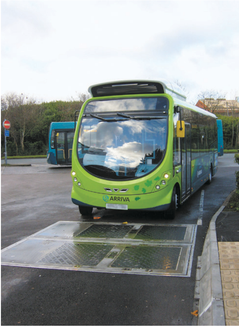
Figure 20.3 An MK electric bus approaches induction charging plates. Photo: Stephen Potter.
