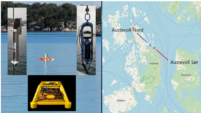
Fig. 3. Pilot demonstrator for environmental oceanographic monitoring at the coast of Austevoll, Norway. The Seaguard and Seabird were deployed in 2022, and the bottom lander is scheduled for deployment in 2023.
