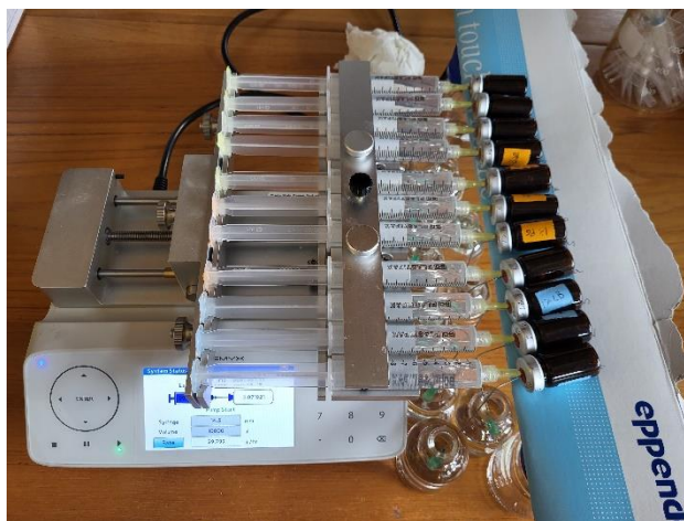
Figure 3.1: Set-up of the syringe pump experiments. In the picture is the Chemyx Fusion 200x with 11 syringes pumping into glass vials with outlet needles leading into narrow neck reagent bottles.
