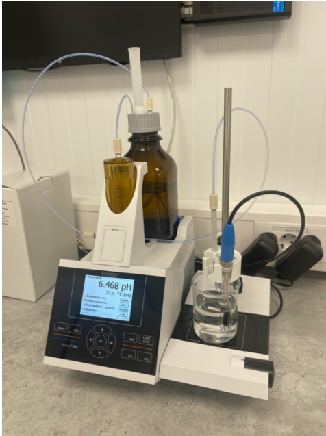
Figure 2.8: The titration machine. The glass beaker is filled with the water sample and the magnetic stir bar is placed in the beaker, along with the pH meter and the pipette containing hydrochloric acid. Picture: (Camilla Dolmen, 2023).
