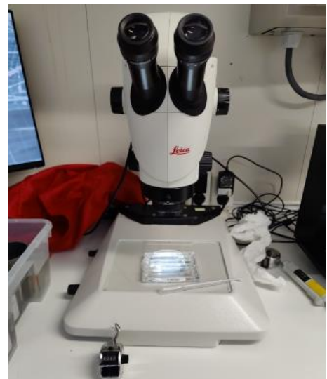
Figure 10: Counting and separating A. tonsa on a zooplankton counting chamber with a pipette under a magnifying glass.
