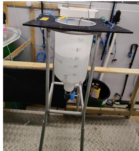
Figure 7: The hatching tank for A. tonsa , with airflow and sensor attached.
