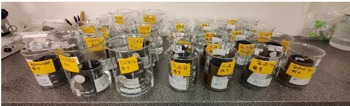
Figure 12: Experimental set up for the preliminary exposure. The first two rows contain the PVC-pipes submerged in their target concentration of Ectosan® Vet. The last two rows contain only filtered sea water.
