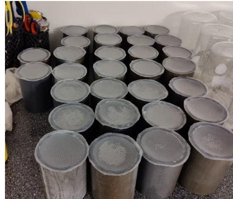
Figure 9: Holding chambers made out of PVC pipes with 50 \mu\text{m} Nitex mesh.
