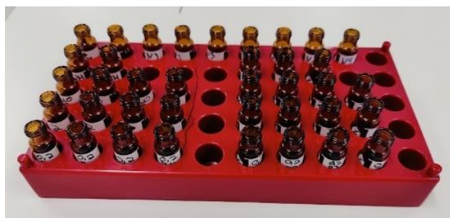
Figure 16: One series with dark vial for each sample, calibration curve, blank without matrix, blank with matrix and controls for one series.
