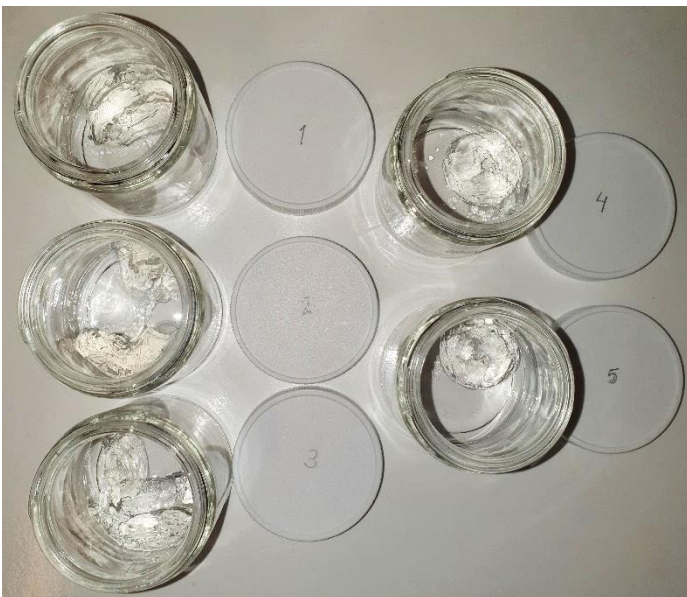
Figure 48: Samples from batch 1 after swelling in distilled water for one week.
