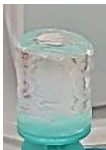
Figure 21: Hydrogel from batch 1 removed from its syringe after 3 days.
