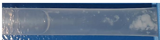
Figure 56: Same sample as in Figure 52, after 1 hour in the pH 9 solution (after 48 hours in pH 4 solution).
