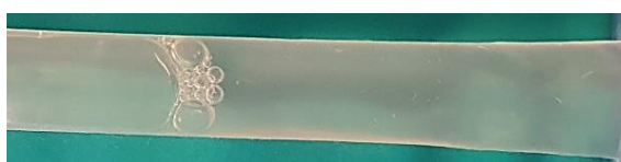
Figure 55: Sample from batch 3 after 48 hours in the pH 4 solution.
