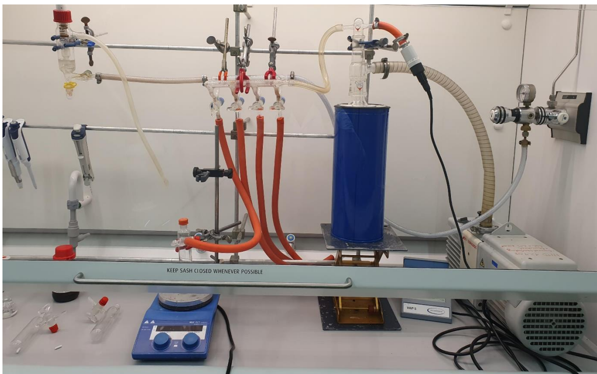
Figure 22: Picture of experiment set-up for batches 3-5, method with Schlenk line.
