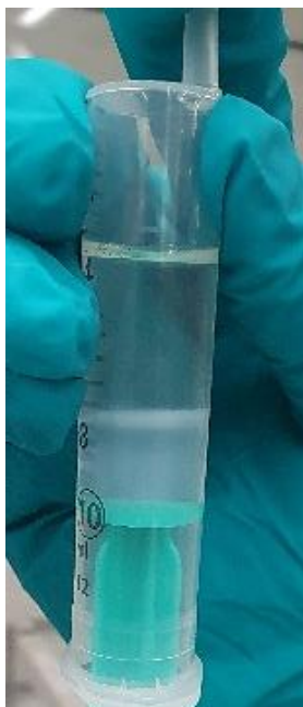
Figure 20: Hydrogel from batch 1 after 24 hours of polymerisation.
