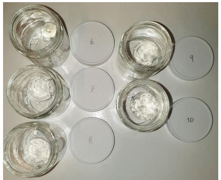
Figure 49: Samples from batch 2 after swelling in distilled water for one week.
