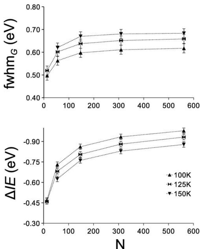
FIG. 6. Calculated mean value ( $\Delta IE$ , bottom) and width ( $fwhm_G$ , top) of theoretical models of S2p photoelectron spectra, plotted against the number of molecules,  $N$ , in the cluster. The clusters were propagated at three different temperatures (100, 125, and 150 K). At each temperature, the uncertainties in calculated  $\Delta IE$  and  $fwhm_G$  values are estimated to 0.02 eV. The effective attenuation length  $\lambda$  is taken to be 10 Å.
