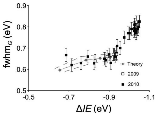
FIG. 7. Comparison of computed and experimentally determined  $fwhm_G$  vs.  $\Delta IE$  values. Computed values are shown for clusters of size  $N = 55, 147, 309$ , and 561, in geometries obtained from molecular dynamics simulations. The upper and lower dashed lines trace values obtained at 150 and 125 K, respectively, with diamonds marking the values obtained as the average of the 125 K and the 150 K data. Estimated error bars have been added to the experimental data points.
