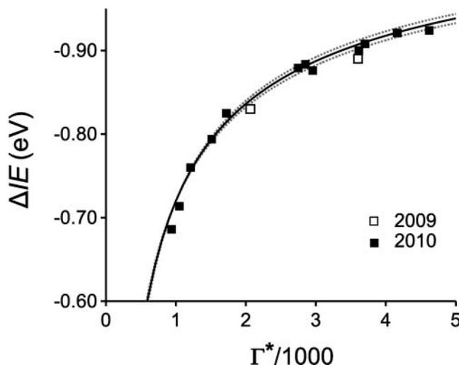
FIG. 5. The cluster-monomer shift in S2p ionization energy,  $\Delta IE$ , plotted against the condensation parameter,  $\Gamma^*$ . The squares show the experimental data points; open (2009) and black (2010). The black solid line represents Equation (3) while the dashed lines indicate the uncertainty associated with the exponential factor in Equation (3).
