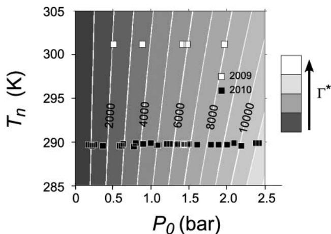
FIG. 1. Contour plot of the condensation parameter ( $\Gamma^*$ ) (Hagena and Obert 1972; Hagena 1981, 1987) as a function of the nozzle temperature,  $T_n$ , and stagnation pressure,  $P_0$ . Experimental conditions are shown as open or filled squares, representing experiments conducted in 2009 and 2010, respectively.
