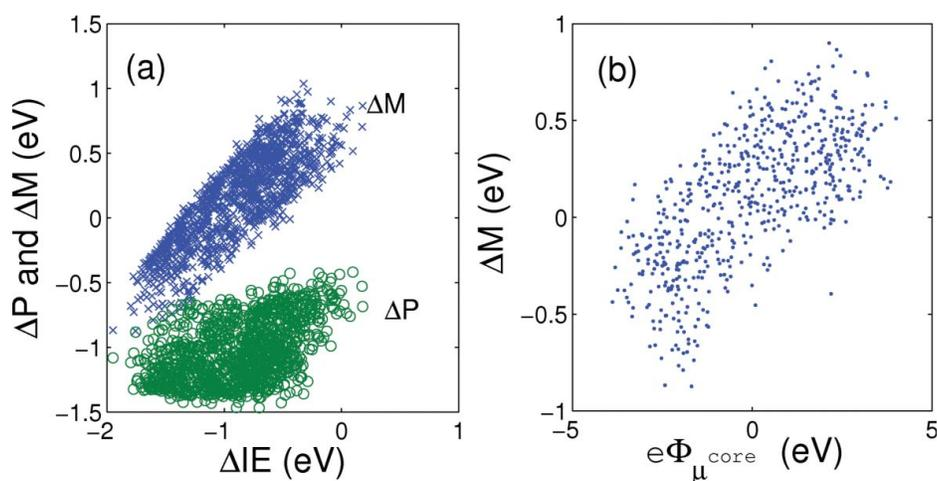
FIG. 10. Analysis of S2p ionization energies (relative to that of the free molecule) for the cluster model described in Figure 9 and in the text. (a) Decomposition of S2p shifts ( $\Delta IE$ ) into contributions from molecular polarization ( $\Delta P$ ) and permanent electrostatic moments ( $\Delta M$ ), and (b)  $\Delta M$  vs. the net dipolar potential at the site of ionization,  $e\Phi_{\mu}^{core}$ , defined by the innermost 20% of molecules frozen to a crystalline core.
