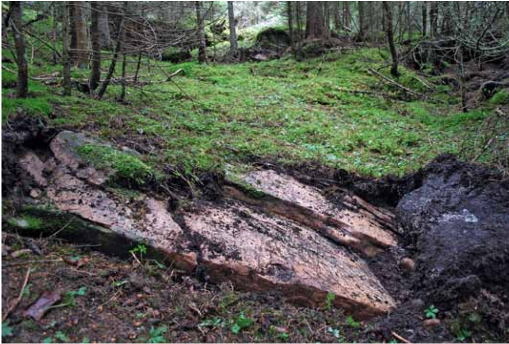
Fig. 5. Part of the old marble quarry at Lænn in Sparbu with its characteristic “plate” structure. Note the simple wedge marks used to break loose material for tombslabs or floor tiles along the cleavage. Photo: P. Storemyr
