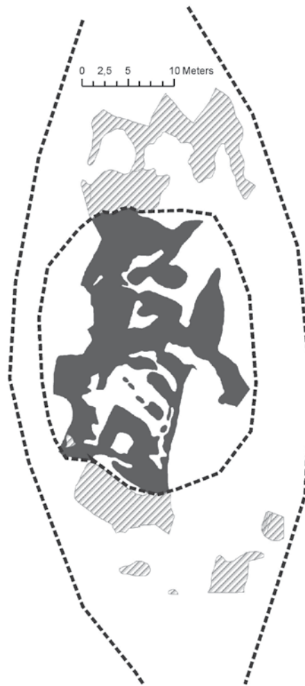
Fig. 4. Map of the Bubakk quarry, Kvikne. Dark grey = serpentinite (core of the deposit). Shaded = soapstone outcrops and quarries. Dotted lines = assumed borders of the rock types. Illustration: T. Heldal
