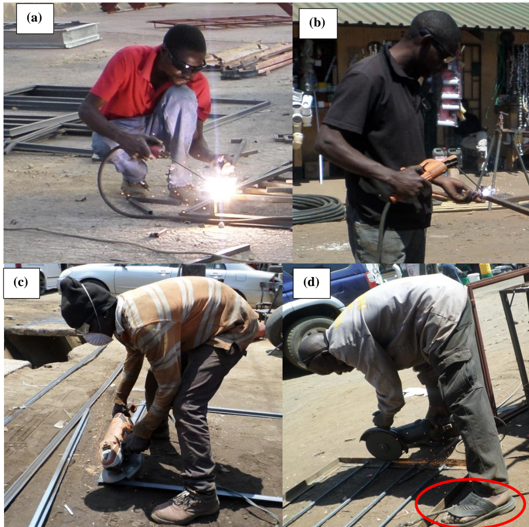
Figure 7: Welding Related Hazards Observed
