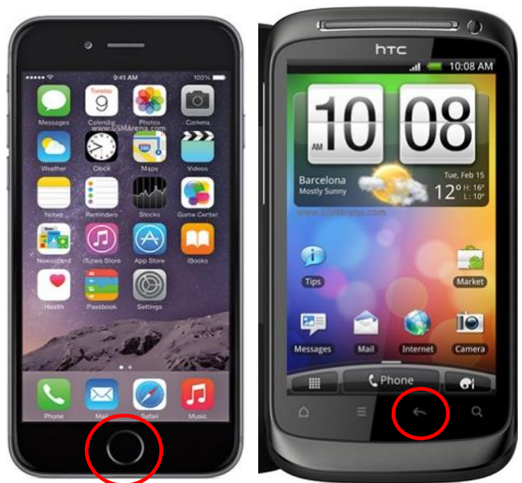
Figure 41 An iPhone with the button that takes you to the home-screen and an Android-phone with the back-button on the bottom.
