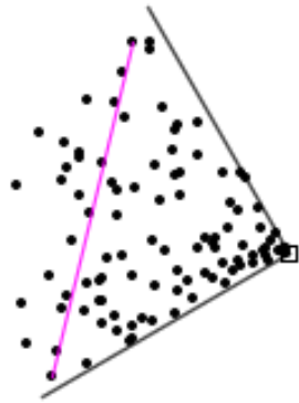
(a) The black square and lines represent the correct cell tower location and cell edges. The black dots represent measurements. The purple line represents l_{direction} .
