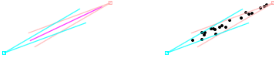
(a) The purple line represents l_{direction} . The blue and pink squares and lines represent the two estimated cell sectors and cell towers solutions.
