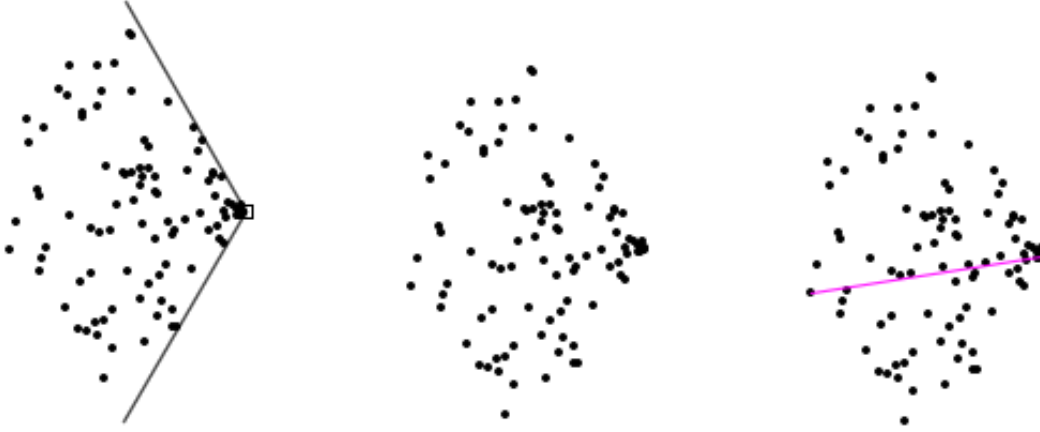
(a) The square represents the cell tower, the two lines represent the cell edges, and the dots represent the measurements. (b) Only the measurements are shown. (c) RSS-DL has computed l_{direction} from the measurements, which is represented by the purple line.
