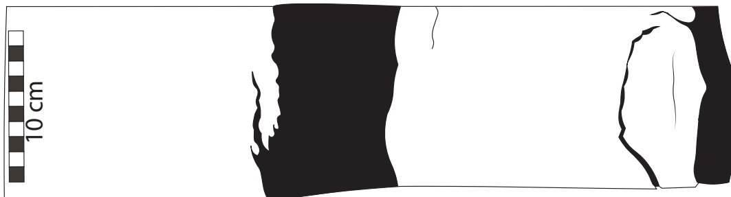
Fig. 21: Illustration of the surface deformation for experiment E4 at \beta 1.37. Side A is in the lower profile plane, side B is in the upper profile plane. The black lines and fields represent displacement surfaces and discontinuities. The scale bar to the left represents 10 cm.
