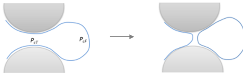
Figure 4-3 Illustration of snap-off using gas injection. A gas bubble penetrates in the narrow throath between two grains (left) and a new bubble is formed (right). P_{cT} is the pressure at the throat, and P_{cF} is the pressure at the leading interface of the gas bubble. Snap-off occurs when P_{cT} > P_{cF} . Reproduced from (Ransohoff and Radke 1988).
