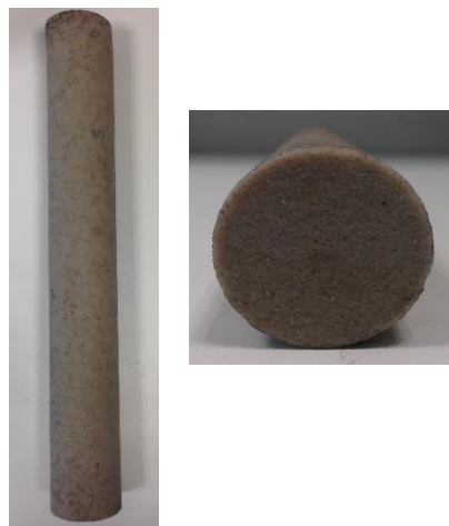
Figure 5-2 Example of sandstone core plug used in the experiment. The core length is 28.8 cm and the diameter is 1.5" (3.8 cm)
