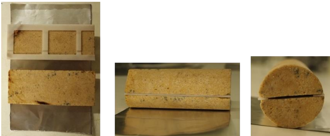
Figure 5-5 Fractured limestone core with POM spacer showing the fracture aperture. One square in the spacer had measured length 3.1 cm, width 2.6cm and thickness 0.1cm. Its total volume was 0.81 cm 3 . The length of the spacer was cut to the same length as the core.
