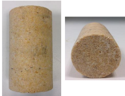
Figure 5-1 Example of limestone core plug used in the experiments. The core length is 7.2 cm and the diameter is 1.5" (3.8 cm)
