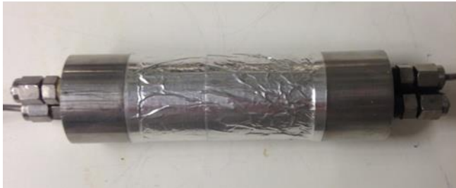
Figure 5-6 (left): Wrapping of core plug in aluminum foil. The core was taped to the core holder end pieces, ready to be assembled in the core holder. (right): Hassler core holder containing core and end pieces ready to be placed in the experimental setup.
