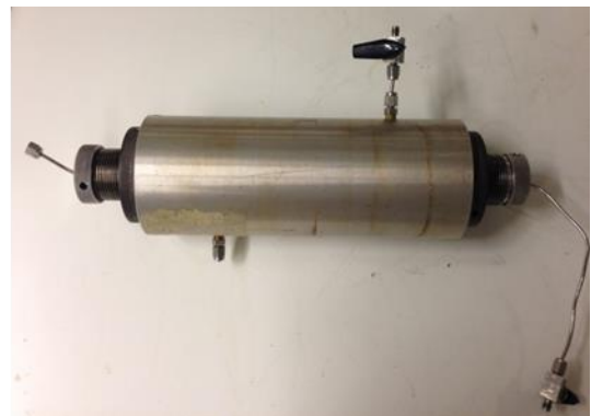
Figure 5-6 (left): Wrapping of core plug in aluminum foil. The core was taped to the core holder end pieces, ready to be assembled in the core holder. (right): Hassler core holder containing core and end pieces ready to be placed in the experimental setup.
