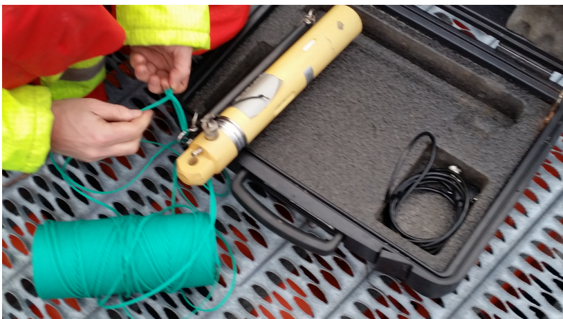
Figure 10. A picture showing the CTD with ropes being attached.
