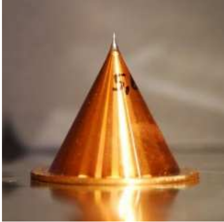
Figure 3.4: shows an image of a glass skimmer with 5.6 \mu\text{m} opening
