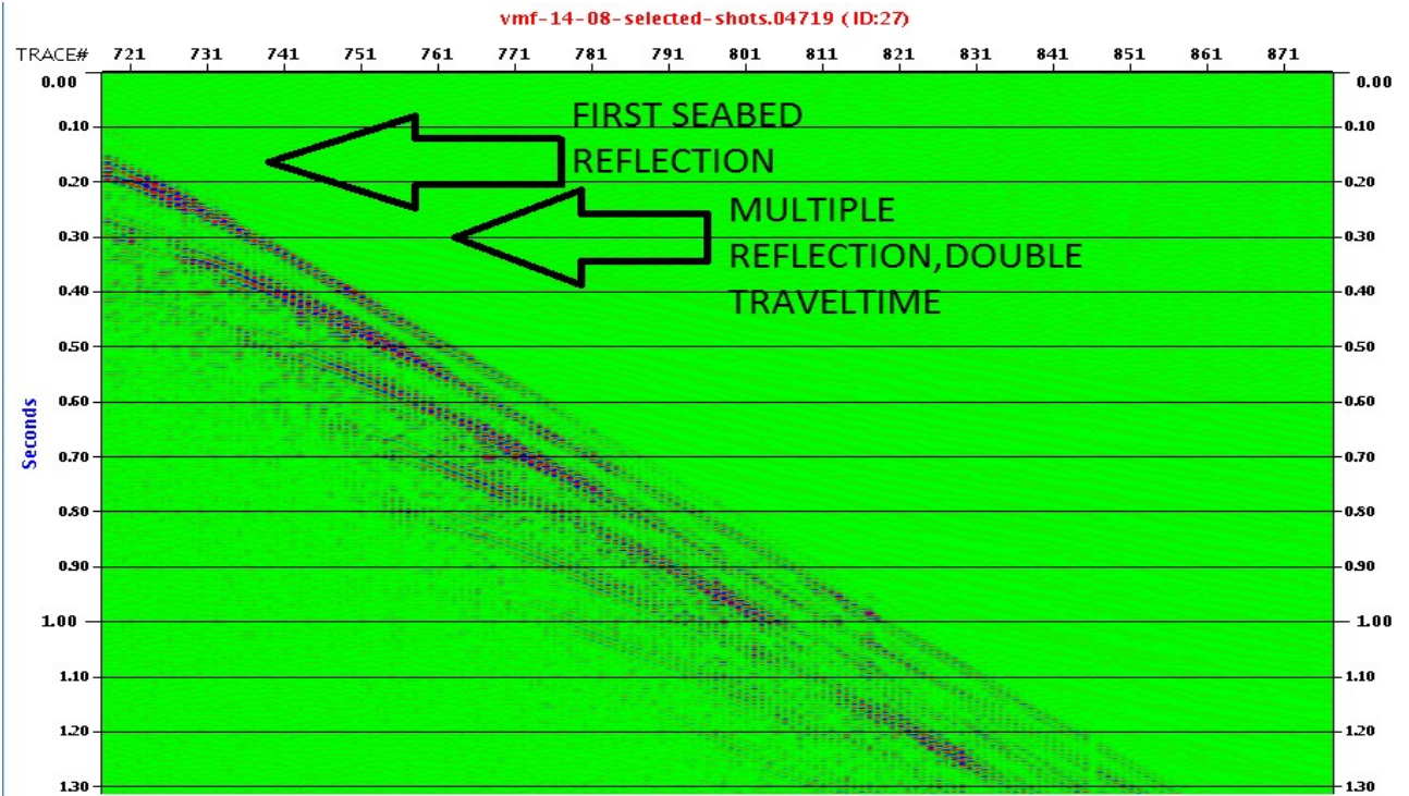
Figure 5.3: The seabed is the first arrow; the second arrow shows the seabed multiple. The shot points are on the x axis and twt in ms is along the y axis.
