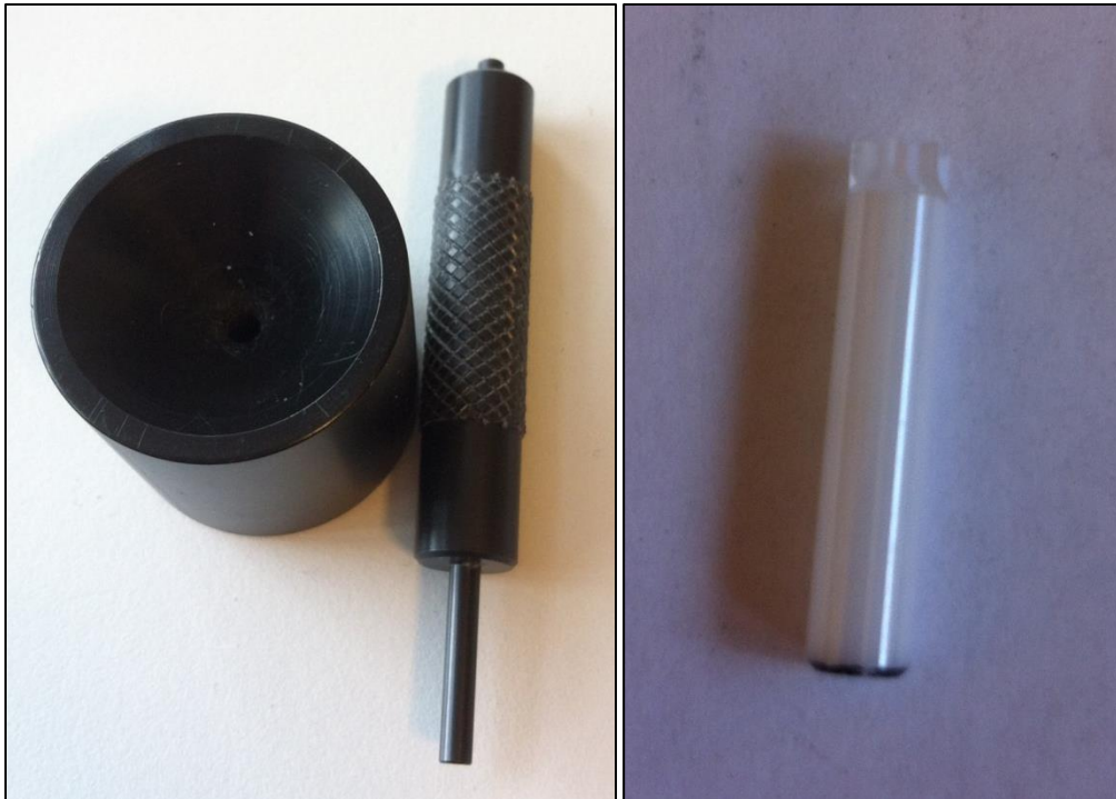
Figure 2.2: Rotor packing rod and funnel (left) and sealed rotor (right). Not to scale.
