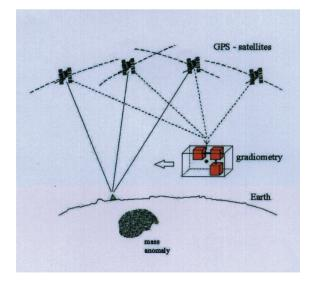
**Figure 3.** Schematic illustration of the principles of combined satellite gradiometry and satellite-to-satellite tracking in high–low configuration (ESA, 1999). \*As for Table 1 we are mostly considering the marine geoid in support of radar altimetry.
