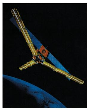
**Figure 2.** Artistic view of the SMOS satellite with the three-legged (4.5 m) passive microwave L-band antenna (Kerr et al., 1999)
