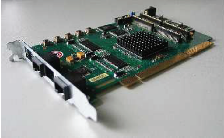
Figure 4.4.: H-RORC data pump and FPGA coprocessor [27].
